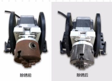
除锈前 Before rust removal 除锈后 After rust removal
